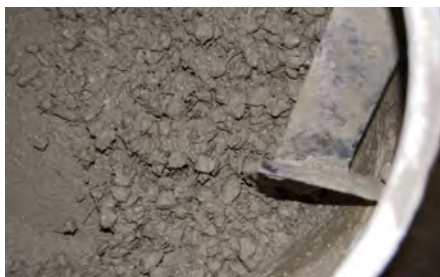
Figure 2. Active Enamel Coated Chopped Metal Wires , or AECCMWs, as thoroughly blended into concrete mix by 3C Inc partner ULRF during Army Phase 1 Program [23]
