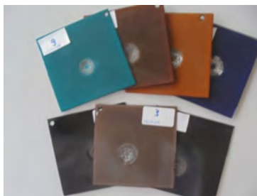
Figure 2. Example of different enamel colors; bond level acceptable to excellent
