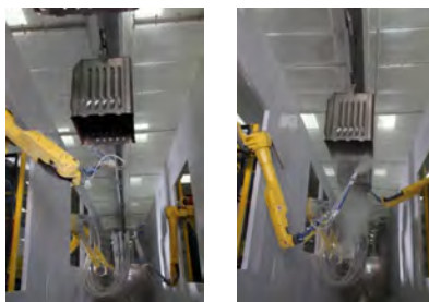
Figure 10. PE powder coating of oven cavities using spray guns integrated with robots
