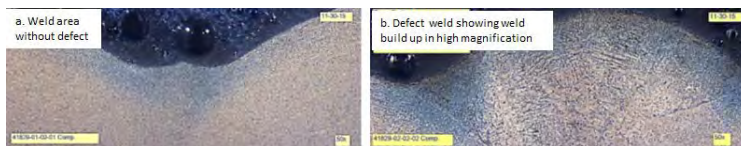
Figure 4. Grain microstructure located in weld area (a) without defect and (b) with the defect
