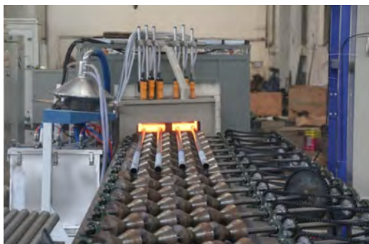
Figure 5. Electrostatic powder enamel application system for extra-long steel pipes
