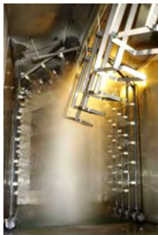
Figure 2. Ideal spray patterns with maximum impingement will optimize the cleaning efficiency
