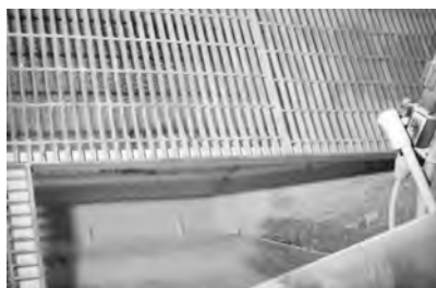
Figure 4. Booth base featured with slopes and fluidizing beds
