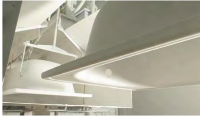
Figure 11. Output of bathtubs from the last, 5th booth after a total application of 1,000 microns of enamel powders
