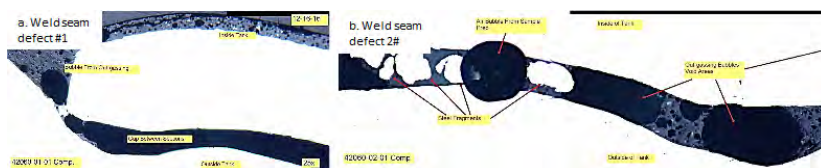
Figure 6. Cross section at weld seam (a) defect #1 and (b) defect #2
