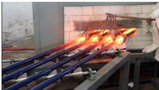
Figure 6. Electric wire pre-heating furnace and medium frequency induction heating system
