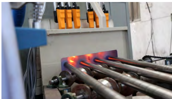
Figure 4. Electrostatic powder enamel application system for extra-long steel pipes
