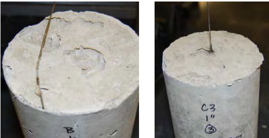
Figure 14. Photos of pullout tests specimens after testing. Left photo is uncoated wire at ½” embedment depth, which pulled out of concrete completely. Right photo is of AECCMF at 1” depth, which left coated wire in the concrete cylinder after completion of the test
