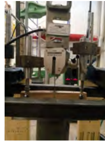
Figure 5. Pullout test specimen in testing apparatus
