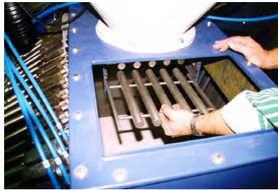
Figure 6. Magnets to remove steel particles from PE powder before transfer into the feed hopper
