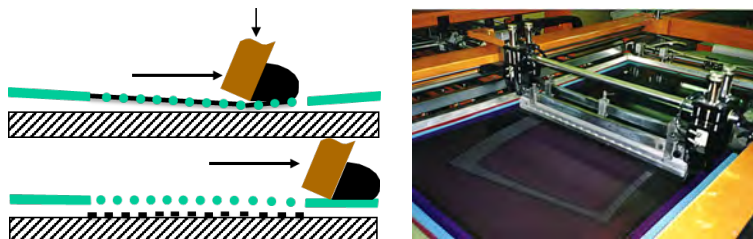
Figure 1. Image of the screen printing process
