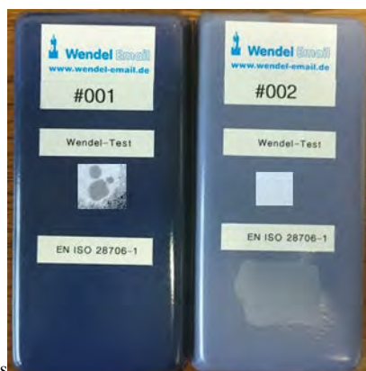
Figure 1. Wendel test results on acid-resistant enamel #001 and non-acid-resistant enamel #002
