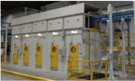
Image 1. Shot blasting machine (courtesy of Pangborn Europe)
