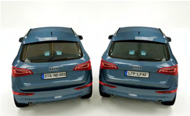
Figure 5. Left, a traditional printing of the window heater and, right, with pre-printed black base
