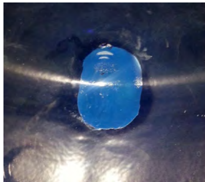
Figure 13. Finished repair 2 ground coat with 30 mils of cover coat.
