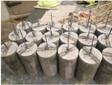
Figure 4. Typical pullout test specimens just after casting
