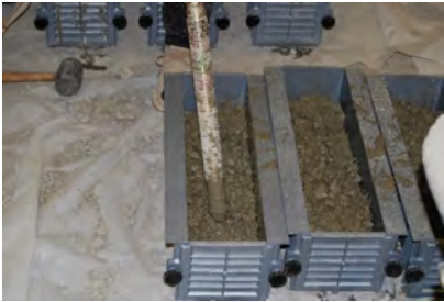
Figure 8. Fiber reinforced concrete added to the beam mold and vibrated; 3% addition
