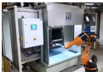
Figure 2. Powder enameling with 6 axis robot i
