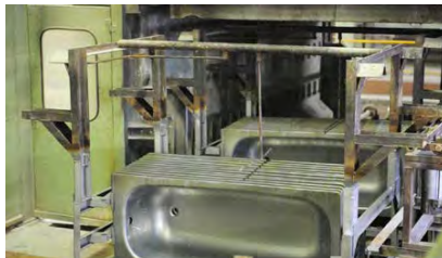
Figures 5, 6 and 7. Line for surface pretreatment with roller track
