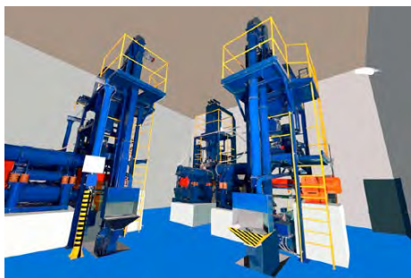
Figure 4. Picture of 2 continuous vibration lines for 500 kg (1,100 pounds) per hour
