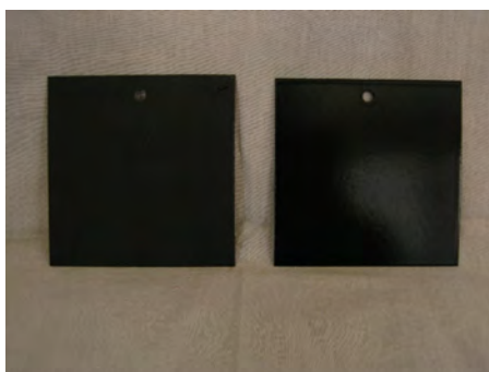
Figure 3. Uncoated substrate on the left and ceramic hybrid coating on the right
