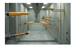
The booth floor is flat and allows easy and safe access for maintenance. Booth walls are available in different materials for every customer need. In robust and wear resistant stainless steel or as plastic sandwich construction. The later is featuring reduced powder accumulation and easier cleaning thanks to their seamless and non conductive surface.
