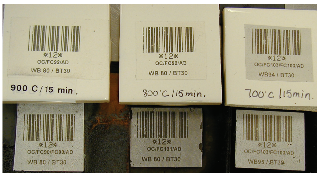
Fig. 3 Pre-ceramic labels on steel (bottom) and ceramic tile (top) after treatment at different temperatures for 15 minutes (from left): 900°C (left), 800°C (middle), and 700°C (right)
