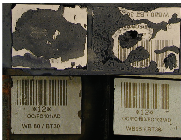
Fig. 2 Pre-ceramic labels on steel plates after 800 °C (left) and 700 °C (right) for 15 minutes respectively: unfilled PSA (top) and filled PSA (bottom)
