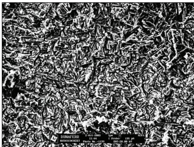
Fig. 8 The surface after pickling of the cold rolled DC04 EK-B grade specimens
