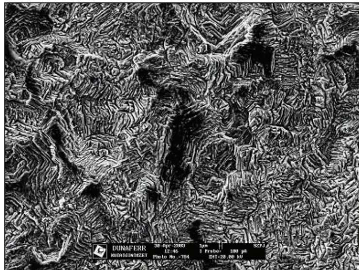
Fig. 7 The surface after pickling of the cold rolled DC04 EK grade specimens
