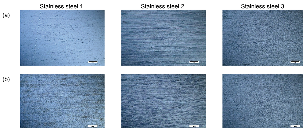
Fig. 3 Microscopic images of surfaces of the stainless steels, 100 x magnified
