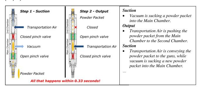
Smart Inline Technology offers significant advantages for the conveying process of enamel powder:
