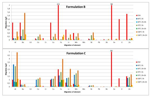
Figure 7: Migration of all elements out of direct on enamel form B and C, compared with DSV
