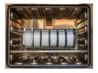
Figure 1: used test equipment to test the migration at 20°C-40°C-70°C (6 migration tests together) and to test the migration into boiling food simulant (test equipment of EN ISO28706-2).
