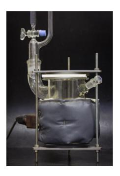
The migration equipment and the food simulants were preheated to the migration temperature before filling. Samples of 15 ml were taken at specific intervals and blanco solution (at the right temperature) was added to ensure the same volume/surface ratio was used. The drop in concentration caused by these samplings (adding the blanco solution) was taken into account.
