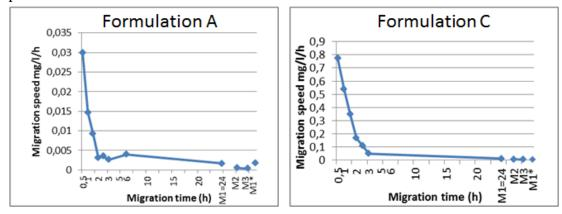
Figure 5:Migration speed of Co out of direct on enamel formulations A and C
