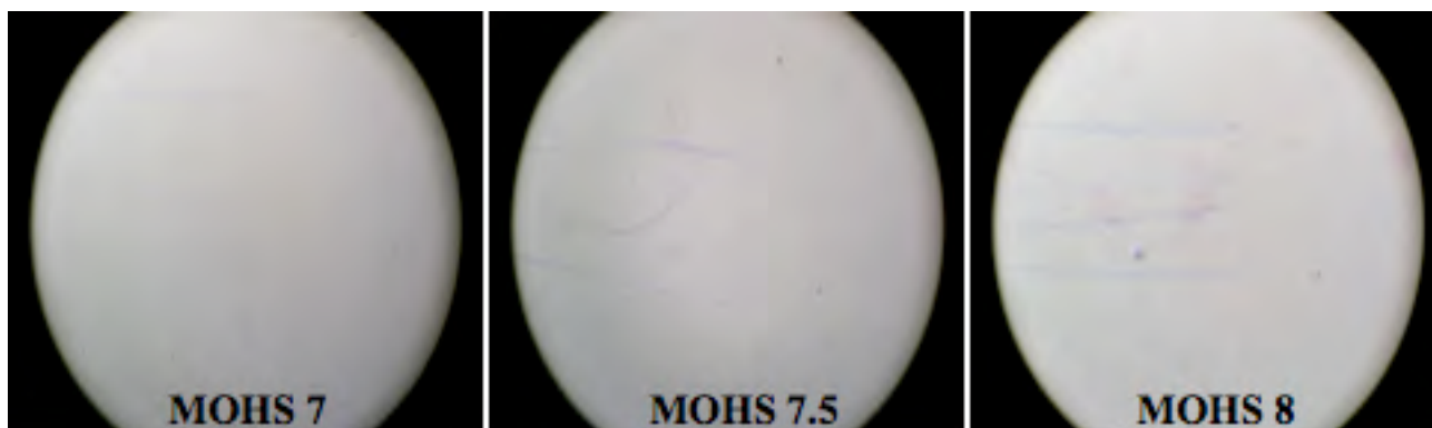
Fig. 22. Results of Mohs anti-scratch test resistance on zirconia treated samples
