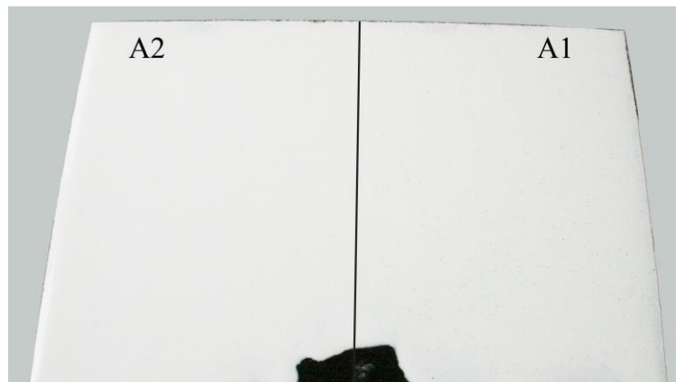
Figure 6: Frits A1 and A2 enameled onto a steel surface with the addition of the cover coat (wet slip application).
