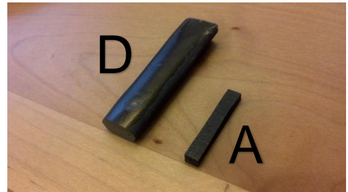
CTE bar D compared for size to machined bar A
