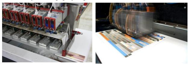
The bar is equipped with "printheads": the apparatus dedicated to the ink application. The printheads have a typical length in the range from 5 to 7 cm.
