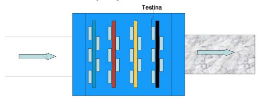
Printers are equipped with an adjustable speed pieces transfer device. A wet enamel should be applied on the pieces, then dried. The temperature of the piece in correspondence of the printheads should not exceed 40 - 45° C to avoid condensation of moisture on the heads or change of the ink viscosity due to the temperature. Both of these phenomena could adversely affect the proper application of the ink.
