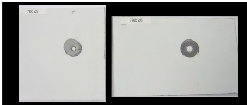
Figure 6 : Adherence of a 2C/1F enamel on degreased steel compared with pre-coated R2E steel (760°C at 0,56 m/min)
