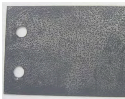
Figure 3 : Enamel without wetting agent (tearing defect)
