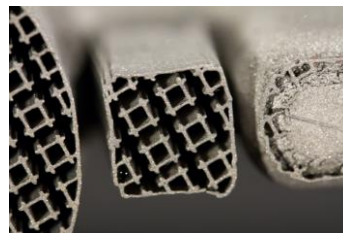
Fig. 12: Support structures on the component are removed mechanically after generative manufacturing.
