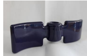
Fig. 13: Agitating element for the THALETEC LabTec-System, manufactured using SLM process and a highly acid-resistant enamel applied. The diameter of the agitating element is 250 mm. Heating and cooling media can flow through the inner cavity.
