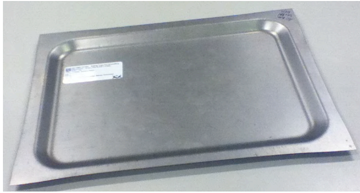
Figure 8 - Geometry of baking tray (overall dimensions: 250 mm x 330 mm)
