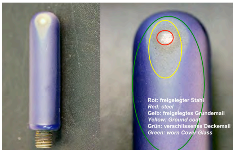
Fig. 7). Whilst the glass lining on the side facing the flow appears dull and worn, the glass lining of the test sample on the other side still has its original shine.
