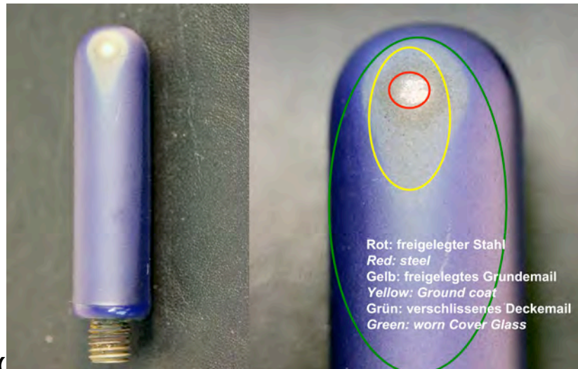
Fig. 7). Whilst the glass lining on the side facing the flow appears dull and worn, the glass lining of the test sample on the other side still has its original shine.
