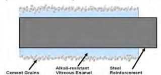
This present study examines effects that can be produced by fusing a porcelain enamel to reinforcing steel surface prior to embedding the steel in a wet concrete structure. This new approach different from previous coating technology in that
