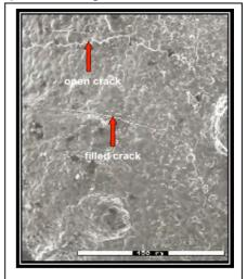
Embedded cement grains hydrate forming calcium silicate gel in fractures
