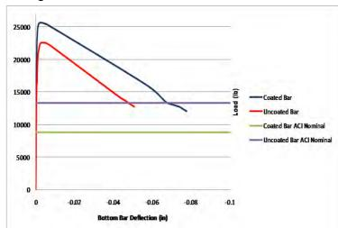
epoxv coated Results of ASTM A994 testing show great improvement in the pullout force as follows: P/E coated rebar 26.1 kips and uncoated rebar 22.7 kips with epoxy coated rebar rated 15.1 kips. The data predict a reduction in required embedment length with P/E coated rebar requiring 15% less
