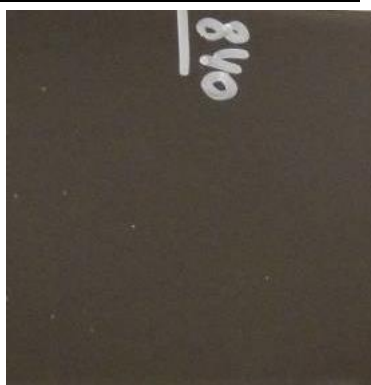
Figure 3: no fishscale appear on grade S390EK after 2-sided enamelling with sensitive enamel (Ferro S43)
