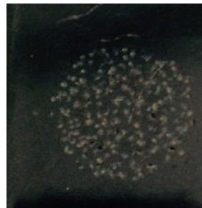
Figure 6: a) Permeation test performed by HELIOS II of ED specimen b) Photo of enamelled sample after test permeation.
